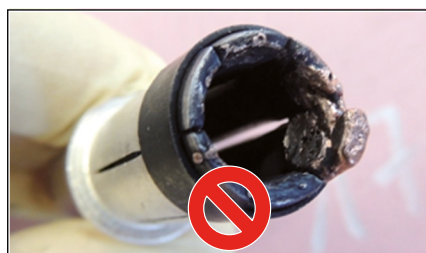
Fig. 13: Socket contact with material covering or removal
