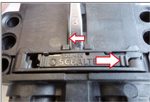
Fig. 5: Move the lock into the unlocked position up to the end stop. Carefully lift the slider with a rotary movement.
