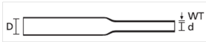
Fig. 1: Heat-shrink tubing, shrink rate 2:1
