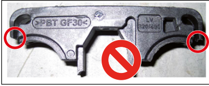
Fig. 24: LV 320/400 S slider with damaged latching hooks
