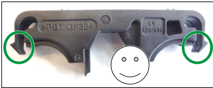
Fig. 23: LV 320/400 S slider with latching hooks that are intact
