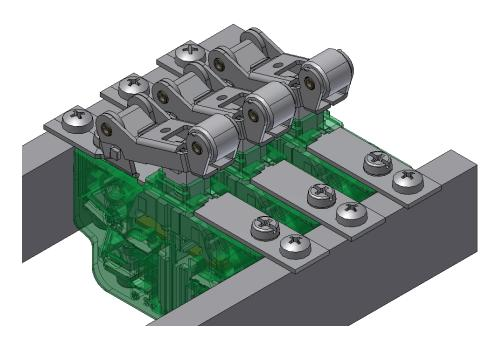
If two circuits are to be switched at once, Schaltbau provides a double switch with a double roller lever for the series S800, S826, S926, S847, S947. To mount two switches, Schaltbau offers a long version of the collar screw that can be ordered with the article description "BS-SK-L", see appendix 8.2.
