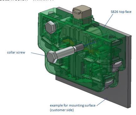
Lateral mounting with a collar screw Ø4 mm with M3-thread (see appendix 8.1) has the advantage that, when correctly tightened, the housing of the switch cannot be mechanically overloaded. This is due to the protrusion of the screw collar, see diagram below.
