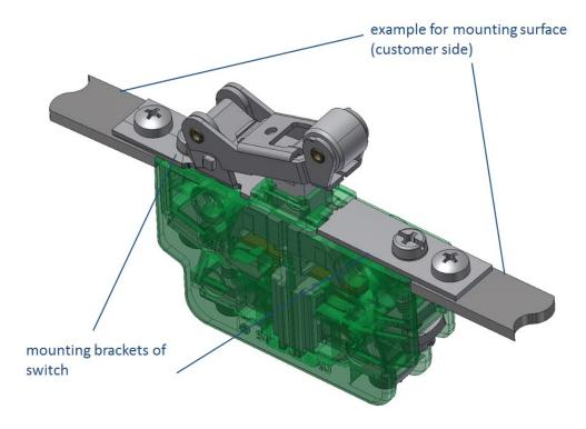
• The two mounting surface holes (customer side) must be adjusted to those of the switches mounting bracket holes.
