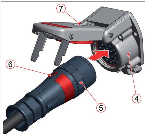
Fig. 21: Align arrow (6) on plug congruent with arrow (7) on the receptacle lid
